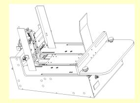
a shuttle type feeder for portable feeding of cards, self-mailers, magazines, etc.
