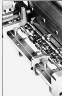
Setting the label stop completes the 2-step width adjustment
