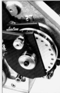
Simple relocation of drive pin sets up the ratchet drive for label width
